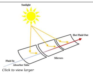
*Figure 1.* Schematic of basic parabolic trough technology.
